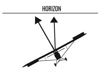
LEVEL THE WINGS FIRST TO REDUCE LOADFACTOR DURING THE PULL UP
